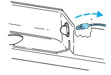
4. Install the bulb socket in lamp assembly by turning it clockwise.
