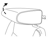
Before returning the seatback to its original position, make sure that cargo or any objects are not trapped behind the seatback. After returning the seatback to its original position, pull on the seatback to ensure that it has fully latched. An unlatched seat may become dangerous in the event of a sudden stop or collision.
