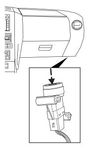
Use the following procedure to reset the fuel pump shut-off switch.
