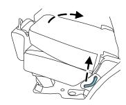
2. Lift up on the head restraint until it locks into its original position.
