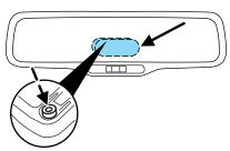
4. Press and hold the reset button on the compass module for approximately 4 seconds until COMPASS ZONE XX appears in the message center display.
