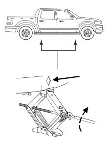
To lessen the risk of personal injury, do not put any part of your body under the vehicle while changing a tire. Do not start the engine when your vehicle is on the jack. The jack is only meant for changing the tire.
