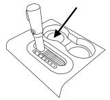
4. Apply the brake and shift into N (Neutral).
