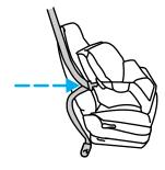
4. Insert the belt tongue into the proper buckle (the buckle closest to the direction the tongue is coming from) for that seating position until you hear a snap and feel the latch engage. Make sure the tongue is latched securely by pulling on it.
