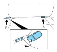
The anchors on the 2nd row outboard seats are provided only to install child seats at the outboard seats. DO NOT install a child seat at the center 2nd row seat using LATCH attachments (rigid or mounted on belt webbing) mounted to the inboard lower anchors at the outboard seats. If you install a child seat at the center 2nd row position, use the vehicle belt and the top tether anchor.
