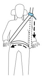
Position the safety belt comfort guide so that the belt rests across the middle of your shoulder. Failure to adjust the safety belt properly could reduce the effectiveness of the safety belt and increase the risk of injury in a collision.
