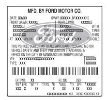
Exceeding the Safety Compliance Certification Label vehicle weight rating limits could result in substandard vehicle handling or performance, engine, transmission and/or structural damage, serious damage to the vehicle, loss of control and personal injury.
