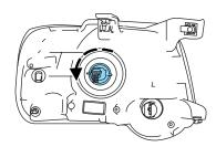
Handle a halogen headlamp bulb carefully and keep out of children's reach. Grasp the bulb only by its plastic base and do not touch the glass. The oil from your hand could cause the bulb to break the next time the headlamps are operated.
