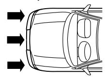
cause activation. Front airbags are designed to activate in frontal and near-frontal collisions, not rollover, side-impact, or rear-impacts unless the collision causes sufficient longitudinal deceleration.
