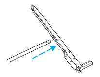
2. Insert the square end of the jack handle extension into the rear access hole located just above the rear bumper and below the tailgate.
