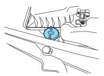
Only use a washer fluid that meets Ford specification WSB-M8B16-A2. Do not use any special washer fluid such as windshield water repellent type fluid or bug wash. They may cause squeaking, chatter noise, streaking and smearing. Refer to the Maintenance product specifications and capacities section in this chapter.
