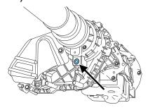
3. Add only enough fluid through the filler opening so that the fluid level is at the bottom of the opening.
