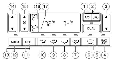
1. **A/C control:** Press to turn on the air conditioning. Press again to turn off the air conditioning. Use
