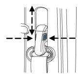
Position the safety belt height adjusters so that the belt rests across the middle of your shoulder. Failure to adjust the safety belt properly could reduce the effectiveness of the safety belt and increase the risk of injury in a collision.
