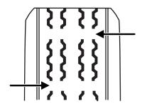
the same height as these "wear bars", the tire is worn out and must be replaced.
