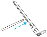
5. Position the jack according to the illustrated guides and turn the jack handle clockwise until the tire is a maximum of 1 inch (25 mm) off the ground.
