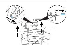
To install the cargo cage, follow the removal procedure in reverse order.
