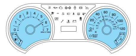
**Speedometer:** Indicates the current vehicle speed.
